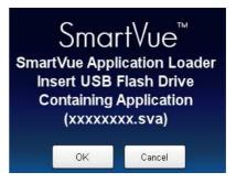
The Application Loader will detect the .sva file and display a message similar to the one shown below.
