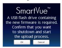
2. Copy the SmartVue application file to a USB flash drive and insert it into the USB port on the back of the unit, then press **OK**. (Pressing **Cancel** will return you to the SmartVue menu without updating the unit.) The SmartVue Application Loader will begin and display the following message:
