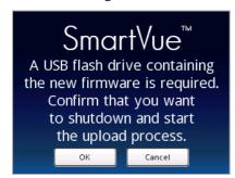
2. Copy the SmartVue application file to a USB flash drive and insert it into the USB port on the back of the unit, then press **OK**. (Pressing **Cancel** will return you to the SmartVue menu without updating the unit.) The SmartVue Application Loader will begin and display the following message:
